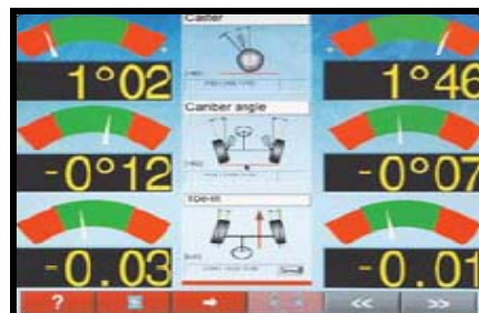
Live front axle alignment readings
